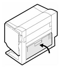
8. Pull the finisher platform about half way out, then loosen the screw on the locking piece (1: viewed from the opposite direction) so that it drops through the slot below it. This keeps the platform from moving while you attach the finisher to it.
